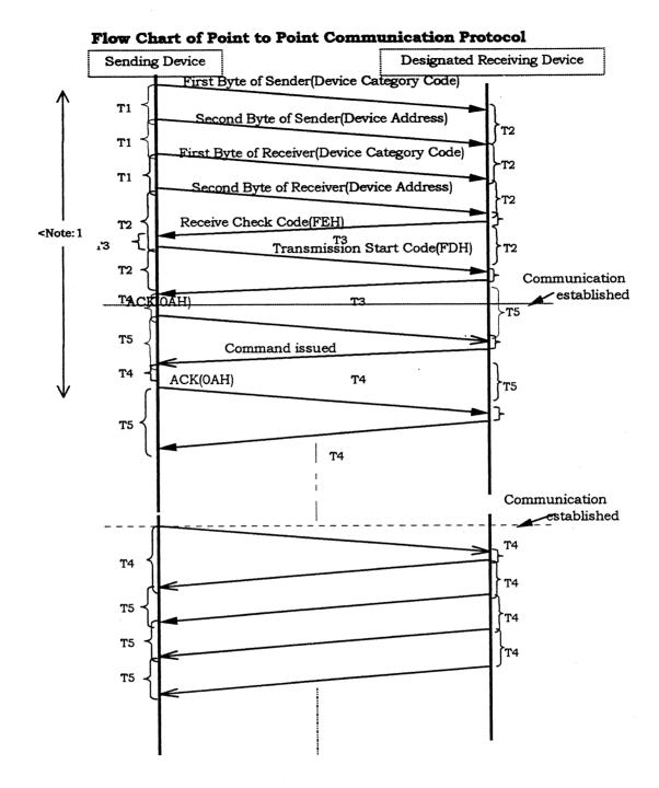
Note: T1(15ms $\Box$ T1 $\Box$ 50ms), T2(T2 $\Box$ 100ms), T3(T3 $\Box$ 50ms), T4(15ms $\Box$ T4 $\Box$ 100ms), <Note:1> T5(T5 $\Box$ 130ms),
